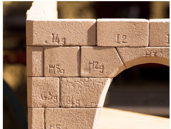
08 Scale model of the prefabrication principle (© M. Valcarce)
