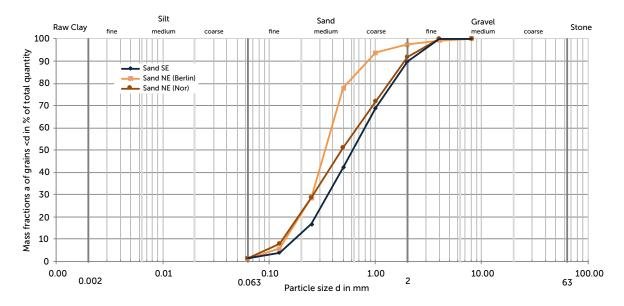
01 Comparison of the particle size distribution for the 0-2 mm fraction
