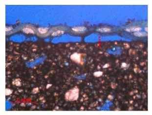
09 Thin section: Detail of the surface zone showing the textile wallpaper, paste d) and earth plaster mortar.
