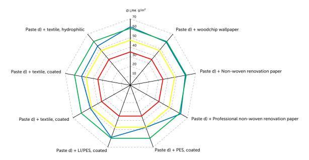
05 Comparison of the sorption activity (12-hour values) of untreated earth plaster mortars (above) with different application systems based on paste d)
