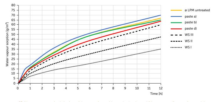
03 Water vapour sorption behaviour of the test surfaces with pre-glued and pasted (blue, green, red) test surfaces and the untreated (yellow) clay plaster mortar samples as well as the water vapour sorption classes WS I to WS III
