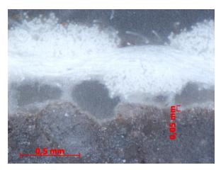
08 Polished section: Detail of the surface zone showing the textile wallpaper, paste a) and earth plaster mortar.
