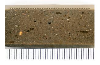
06 Polished section of a composite specimen of earth plaster, textile fabric, glued on flat with cellulose paste
