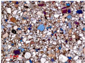
07 Thin section, 35 μm thick, showing parallel polarizers, a little binder (clay constituents), high quartz content and high open porosity
