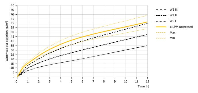
01 Water vapour sorption behaviour (mean value of 20 individual measurements) for untreated earth plaster mortar samples with minimum and maximum values (yellow) compared against the water vapour sorption classes WS I to WS III (black dashed lines)
