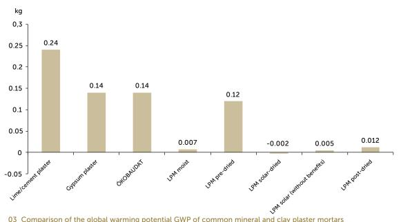
03 Comparison of the global warming potential GWP of common mineral and clay plaster mortars
