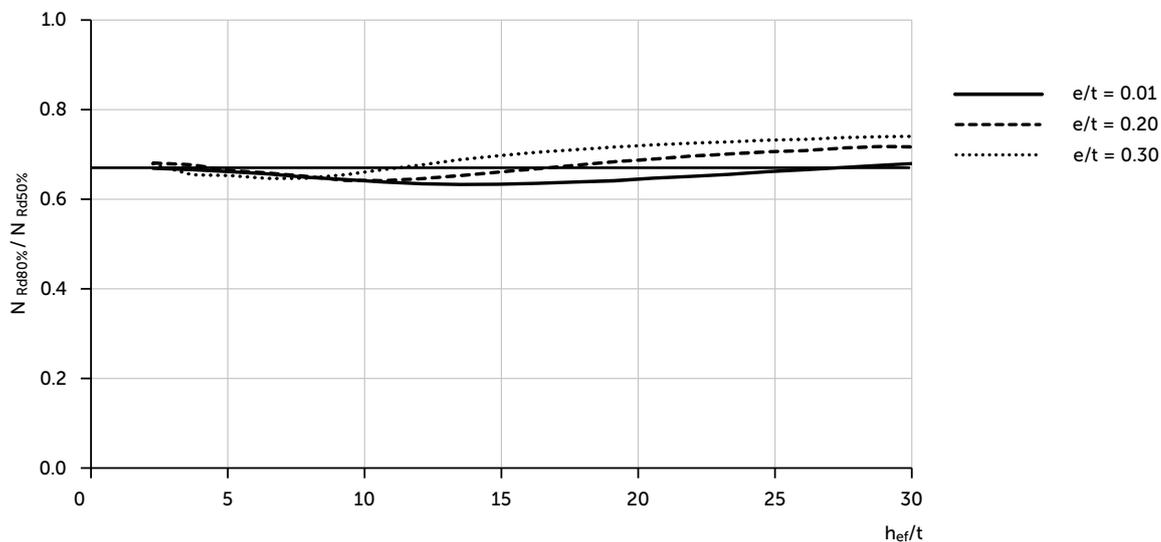
12 Ratio of load capacity at 80% RH to load at 50% RH
