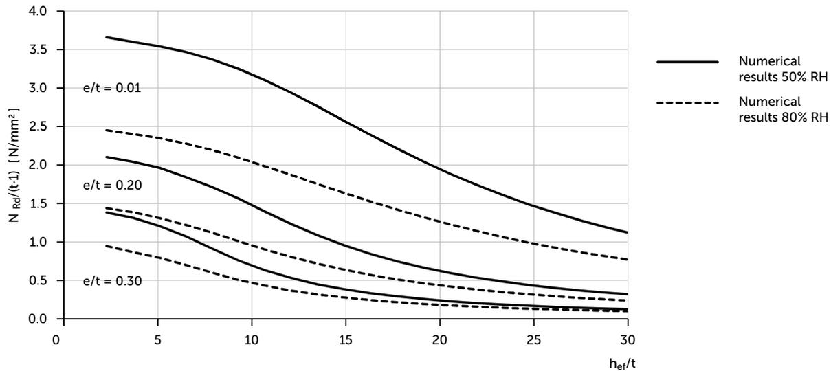
11 Numerically determined bearing capacity of earthen masonry under eccentric compressive load at 50% RH and 80% RH
