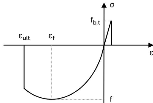
09 Total strain crack model of the masonry blocks
