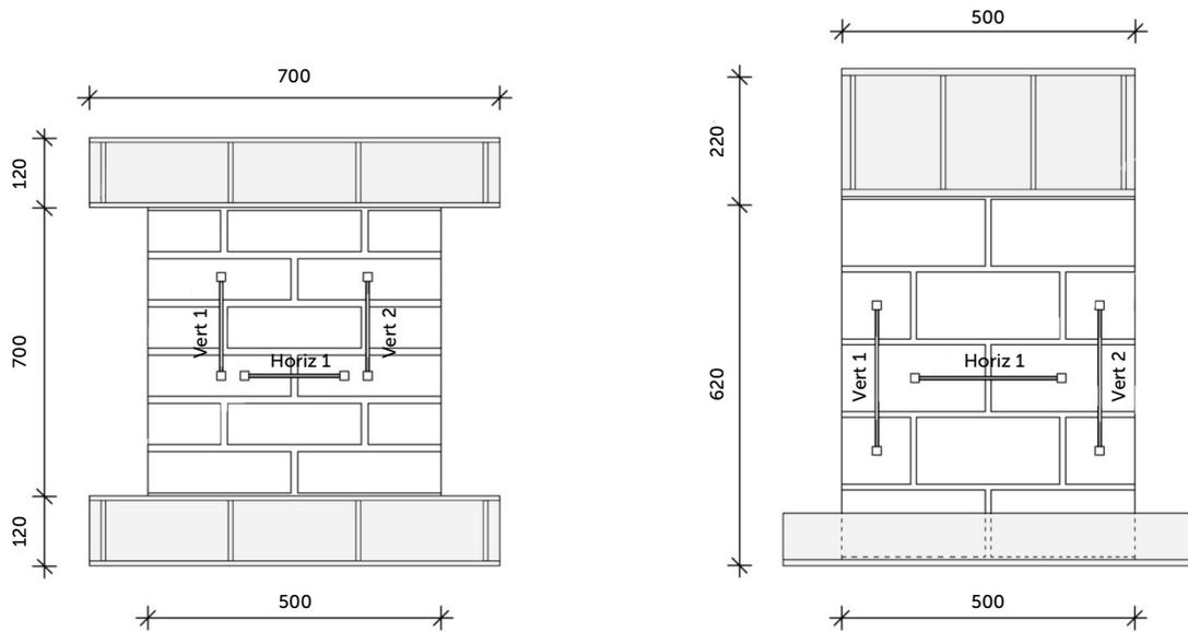
03 Layout and length of the measuring sections of the RILEM test specimens taken from NF blocks (a) and 3DF blocks (b)
